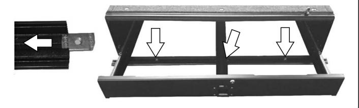
( **E** ) Looking at the rear of the Drawer System, remove the bolts as indicated by the arrows. Keep the bolts and washers safe as they will be used at a later stage.
