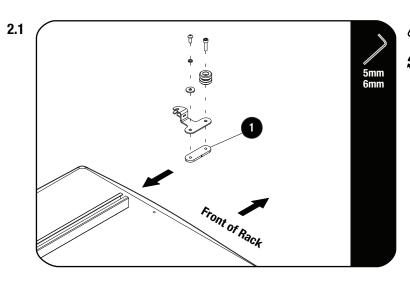
Before assembling the Channel Nut Plate (Item 1), refer to TBMK012 fitment guide.
