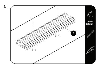
Determine the best possible postion for mounting the Tracks (Item 1). Take care not to drill into or "through" any reinforcements.
