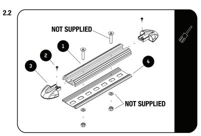
Use suitable M6 Fixings (Not Supplied) to secure the Tracks (Item 1) to the roof. The Tracks and Protective Trim (Item 4) must be used on the roof.
