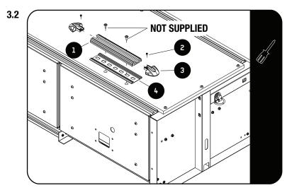
Use suitable M6 Wood Fixings (Not Supplied) to secure the Tracks (Item 1) to the Drawer System. The Tracks and Protective Trim (Item 4) must be used on the Drawer System.
