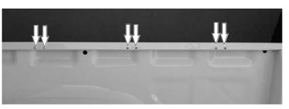
( **E** ) Ensuring that the Rubber Track Liner (Item 5) is fitted to the Tracks, reposition each Track lining up the holes in the Track with the holes from Step 2D. Insert the M6 x 25 Countersunk Bolts (Item 2). Place the Clamp Plates (Item 6) behind the lip on the load bed and over the ends of the Countersunk Bolts. Secure the Clamp Plate and Track in position using the M6 Flat Washers and M6 Nyloc Nuts (Items 7, 8).
