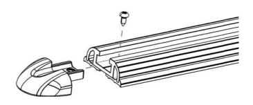
(  ${f B}$  ) Fit a Plastic End Caps received with your Load Bars into each end of the Load Bars as shown.
