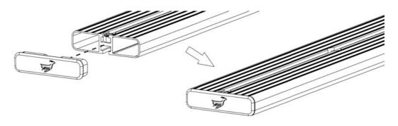
( C ) With the Load Bars in the upside down position (Check using the Buck Logo on End Caps from Step 2B as an indicator), slide two M8 x 25 Hex Bolts supplied with the Universal Load Bed Legs into each end of the Load Bars using the machined slots as shown.
