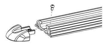
(  ${f B}$  ) Fit a Plastic End Caps received with your Load Bars into each end of the Load Bars as shown.
