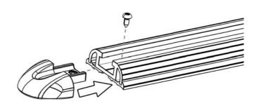
( **D** ) Grab your friend and with one of you on each side of the Rack, flip it end over end so that the bolts are facing down. Approach the vehicle from the rear lifting the Rack above the Legs. Slowly lower the Rack lining up the bolts in the Rack with the holes in the Legs. You may need to adjust the position of the Legs.
