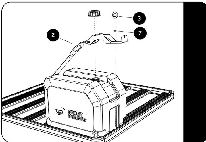
The Tank may be taken off the Rack by removing the Plastic Cap, loosening the M8 Eye-nut and lifting the Tank Strap up and over as shown.
