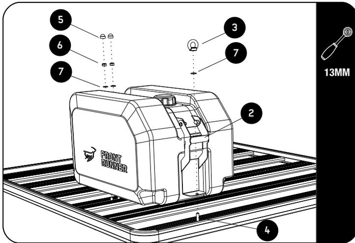
Place the Tank with Tank Strap (Item 2) onto the Rack as shown, lining up the holes in the Tank Strap with the Hex Bolts inserted in Step 2.2 and 2.3. Ensure that the Tank is sitting centered on the T-Slot Beading and secure the Strap to the Rack using the M8 Eye Nut, M8 Flat Washer and M8 x 30 Hex Bolt (Items 3, 4 & 7) as shown.
