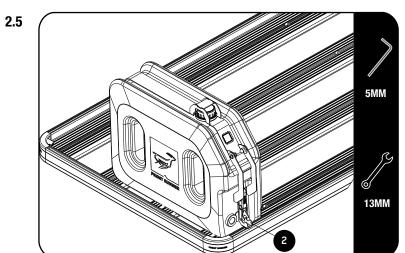
Open the Strap and place the Pro Water Tank onto the rack. Close the Strap over the Water Tank as show.
