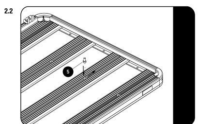
Slide the M8 x 16 Hex Bolt (Item 5) into the 3rd slats machined slot as shown.
