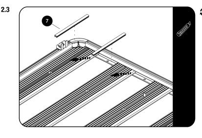
Cut the T-Slot Rubber (Item 7) in two equal lengths before inserting it into the slats T-slot as shown.
