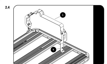
Loosely fit the Pro Tank Strap (Item 1) to the rack using the M8 x 16 Hex Bolt from 2.3 and M8 Nyloc Nut (Item 4) as shown.
