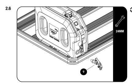
Before fitting the Tap (Item 9) apply thread tape to the thread of the tap.
