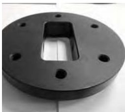
Fig. 3: Correct bolt pattern has no dot marking
