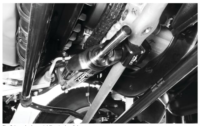
Fig. 2: Loosely clamp stabilizer to drag link.
