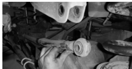
Fig. 1: Track bar removal
