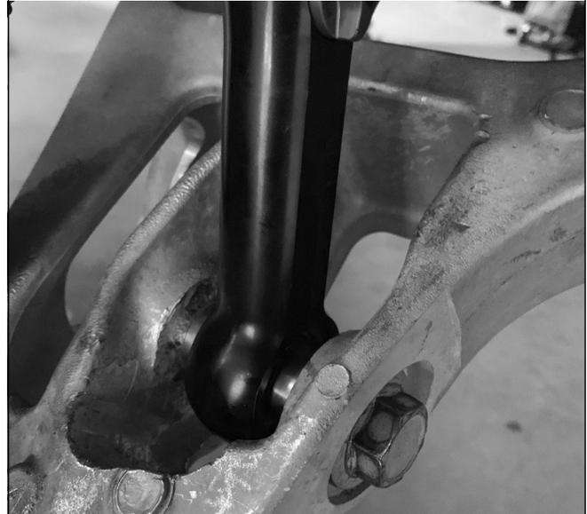
**Note: The user can clock the eyelet with the switch facing away or towards the front of the truck. Rotate the eyelet to have the switch face the back of the truck if desired.**
