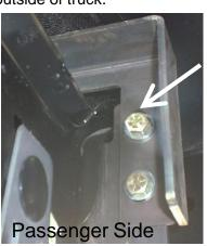
**Step 3:** (EDDIE BAUER EDITION ONLY: Remove lower bumper grille so that upper bracket can stick through bumper! Grille can be cut and reattached after install depending on customer). Attach upper support bracket to the side of frame horn bracket that was bolted on in step 2 using supplied bolts. The angle in the bracket should face the inner side of truck.
