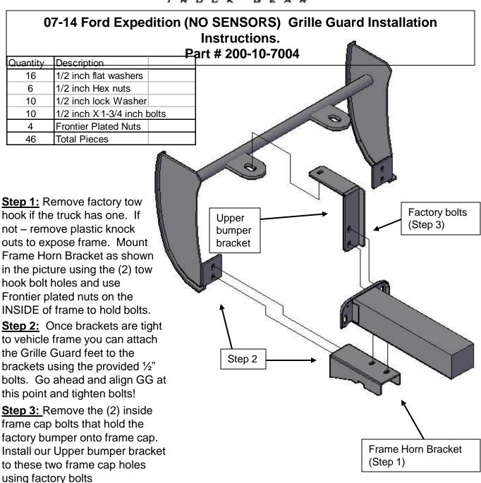
upper bumper brackets. Grille guards tabs will attach UNDER upper bumper bracket.
