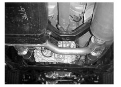
INSTALL Y-PIPE # A ONTO YOUR EXISTING STOCK FLANGES. INSERT HANGER INTO RUBBER GROMMET. USE YOUR FACTORY HARDWARE TO SECURE. DO NOT TIGHTEN.
