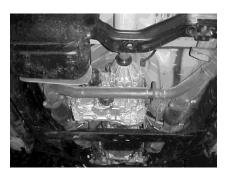
LAY OUT THE GIBSON EXHAUST ON THE FLOOR AND COMPARE PART #'S TO THE DRAWING. TO REMOVE THE STOCK EXHAUST REMOVE IT FROM THE 2 BOLT FLANGES, LOCATED IN FRONT OF YOUR FACTORY MUFFLER. NEXT, CUT IFF YOUR STOCK TAILPIPE BEHIND YOUR MUFFLER. DO NOT DISGARD YOUR FACTORY HARDWARE, YOU WILL RE-USE IT.
