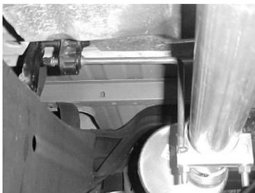
INSTALL MUFFLER #B ONTO HEADPIPE 1-1/2" TO 2" WITH INLET TOWARDS THE ENGINE. OUTLET SHOULD BE AT THE 2 O'CLOCK POSITION. USE CLAMP #E AND #F TO SECURE MUFFLER TO THE HEADPIPE, INSERT MUFFLER HANGER INTO RUBBER GROMMET. DO NOT TIGHTEN. THE INLET OF THE MUFFLER IS LOOKING INTO THE LOUVERS.
