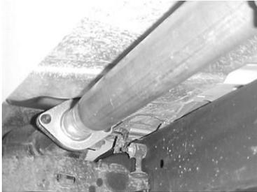
TO REMOVE STOCK EXHAUST UN-BOLT IT FROM THE 2-BOLT FLANGE LOCATED BETWEEN THE CATALYTIC CONVERTER AND THE MUFFLER. NOW CUT OFF YOUR STOCK TAILPIPE JUST BEHIND THE MUFFLER AND REMOVE. LEAVE ALL RUBBER GROMMETS ON THE HANGER. USE WD-40 TO AID IN REMOVAL OF EXHAUST AND HANGERS. INSTALL HEADPIPE #A, USE # G GASKET, AND RE-USE YOUR FACTORY BOLTS. DO NOT TIGHTEN.
