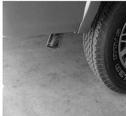
INSTALL YOUR STAINLESS TIP. TO CLEAN TIP USE ANY STAINLESS OR ALUMINUM CLEANER AND A SCOTCH BRITE PAD. NOW GO BACK AND TIGHTEN ALL CLAMPS, BOLTS AND NUTS.
