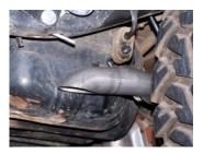
7. Adjust tailpipe to best fit your vehicle. Tighten all clamps and flanges working your way from the front to the back.
