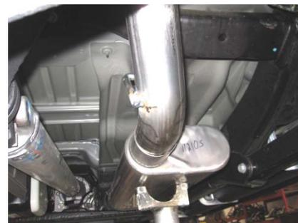
4. Install over axle pipe Item # C into the muffler outlet. Slip the hangers into the rubber grommets and keep tailpipe loose use clamp #E to secure together.
