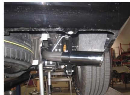
7. Be sure to check all clearance after each section has been tightened to be sure there is proper clearance. It may take 4-500 miles for your vehicle to fully adjust to the changes in exhaust flow.
