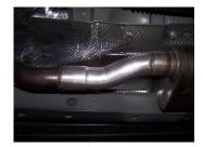
3. Install headpipe #A onto your existing stock front pipe and attach with clamp #E. Do not tighten.
