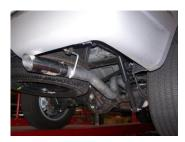
6. Slide the over axle tailpipe #C into the muffler 1.5-2". Secure pipe to muffler using clamp #E. Do not tighten. Insert welded hangers into rubber grommets.
