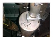
4. Slide muffler #B over headpipe 1.5-2" with louvers facing towards the converter. Use a jack stand to support the muffler. Use clamp #E to secure muffler to headpipe. Do not tighten. Outlet should be at the 1 o'clock position.
