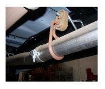
1. LAY OUT THE EXHAUST SYSTEM SO IT MATCHES THE DRAWING. MAKE SURE ALL PART NUMBERS ARE CORRECT. UNBOLT THE WELDED MUFFLER ASSEMBLY IN FRONT OF THE MUFFLER. DO NOT REMOVE THE **EXTENSION PIPE BEHIND** THE CONVERTER. FOR AN EASIER REMOVAL OF THE FACTORY EXHAUST. CUT THE TAILPIPE JUST BEHIND THE FACTORY MUFFLER. LEAVE ALL RUBBER GROMMETS IN PLACE. USE WD-40 FOR EASIER REMOVAL OF FACTORY HANGER.
