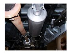
3. INSTALL MUFFLER #B. THROUGH BAND CLAMP THEN SLIDE ONTO HEADPIPE 1½" TO 2". USE CLAMP #E TO SECURE MUFFLER TO HEADPIPE.
