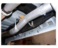
2. INSTALL HEADPIPE #A ONTO THE FACTORY EXTENSION PIPE. INSERT WELDED HANGER INTO RUBBER GROMMET. USE CLAMP #E TO ATTACH IT TO THE FACTORY EXTENSION PIPE. DO NOT TIGHTEN
