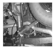
INSERT WELDED HANGER INTO THE RUBBER GROMMET.
