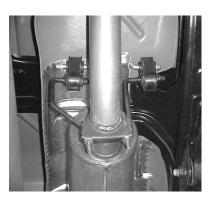
INSTALL HANGER #G ON THE OUTLET OF THE MUFFLER. DO NOT TIGHTEN.
