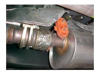
Lay out the exhaust on the floor so it looks like the drawing and compare parts with manual. To remove the stock exhaust Remove from the 2-bolt flange in front of your stock muffler. Also remove exit pipe from the clamp at the rear. Cut off tailpipe just after the muffler. Leave all rubber grommets in place. Use WD-40 to aid in removal of exhaust and hangers. Do not discard your factory hardware, for you will re-use it.
