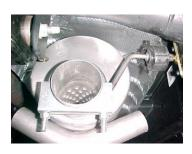
Install muffler #B onto head pipe 1-1/2" to 2" with the louvers facing towards the converter. Outlet will be at the 6 o'clock position. Use a jack stand to support the muffler. Use clamp #E to secure the muffler to the head pipe. Do not tighten. Muffler inlet is looking into the louvers. Next, install rear muffler hanger #F onto muffler outlet. Insert hanger into rubber grommet.
