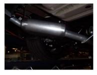
3. Install passenger side muffler assembly #B. Insert welded hangers into rubber grommets. Use clamp #D to secure pipes together. Do not tighten.
