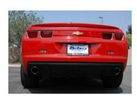
6. When you have everything in place, firmly tighten all bolts and clamps down securely. Inspect all fasteners after 25-50 miles of operation and retighten as necessary.
