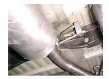
SLIP THE OVER AXLE TAILPIPE #C INTO THE OUTLET OF THE MUFFLER 1-1/2" TO 2". CONNECT REAR HANGER TO FACTORY MOUNT LOCATED AT THE REAR OF THE VEHICLE WITH FACTORY BOLT. INSERT WELDED HANGER INTO RUBBER GROMMET. USE CLAMP #E TO SECURE TAILPIPE TO THE MUFFLER. DO NOT TIGHTEN.
