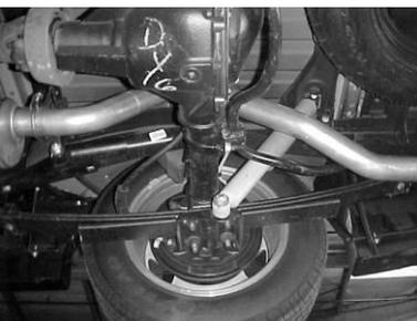
INSTALL OVERAXLE TAILPIPE #C INTO MUFFLER AT LEAST 1 1/2" TO 2". SHORTER END GOES IN TO MUFFLER. SPARE TIRE MIGHT HAVE TO BE LOOSENED AND PUSHED OVER TOWARDS THE DRIVERS SIDE FOR BETTER CLEARANCE. ATTACH TO CLAMP # H.
