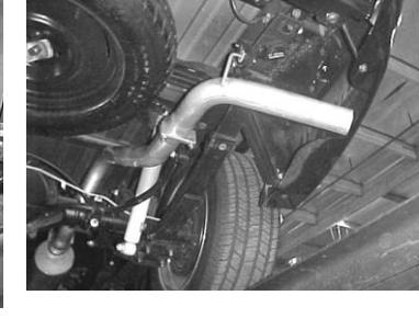
INSTALL TURNOUT PIPE #D & INSERT WELDED HANGER INTO THE RUBBER GROMMET. USE CLAMP #G TO SECURE TAILPIPE TO THE OVERAXLE PIPE. DO NOT TIGHTEN
