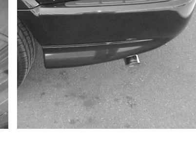
INSTALL STAINLESS TIP. USE ANY STAINLESS CLEANER TO CLEAN TIP. YOU CAN NOW TIGHTEN ALL NUTS, BOLTS, FLANGE AND CLAMPS STARTING FROM THE FRONT AND WORKING YOUR WAY TO THE BACK
