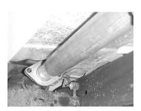
TO REMOVE STOCK EXHAUST **UN-BOLT IT FROM THE 2-BOLT** FLANGE LOCATED BETWEEN THE CATALYTIC CONVERTER AND THE MUFFLER. NOW CUT OFF YOUR STOCK TAILPIPE JUST BEHIND THE MUFFLER AND REMOVE. LEAVE ALL RUBBER GROMMETS ON THE HANGER. USE WD-40 TO AID IN REMOVAL OF EXHAUST AND HANGERS. INSTALL HEADPIPE #A, USE #G GASKET, AND RE-USE YOUR FACTORY BOLTS. INSERT WELDED HANGER INTO RUBBER GROMMET. DO NOT TIGHTEN.
