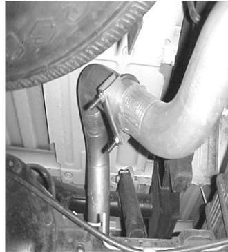
SLIP OVERAXLE TAILPIPE #D INTO THE OUTLET OF THE MUFFLER NO LESS THAN 1 1/2" AND NO MORE THAN 2". ATTACH CLAMP #F AT THE MUFFLER OUTLET (**DO NOT TIGHTEN**). INSERT WELDED HANGER INTO RUBBER GROMMET.
