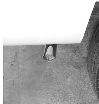
INSTALL YOUR STAINLESS STEEL TIP. NOW TIGHTEN ALL CLAMPS AND RE-INSTALL THE O2 SENSOR INTO THE PASSENGER SIDE HEADPIPE. WE RECOMMEND USING ANTI-SEIZE ON ALL THREADS. USE ANY ALUMINUM OR STAINLESS STEEL CLEANER TO POLISH YOUR TIP.
