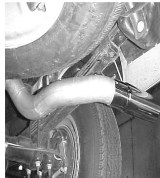
INSTALL TURNOUT PIPE #E. INSERT WELDED HANGER INTO RUBBER GROMMET. ATTACH CLAMP #F TO CONNECT TAILPIPE TO TURN OUT PIPE. (**DO NOT TIGHTEN CLAMP**) ADJUST TURNOUT PIPE SO IT EXITS ON THE SIDE OF THE VEHICLE AT A LEVEL POSITION.
