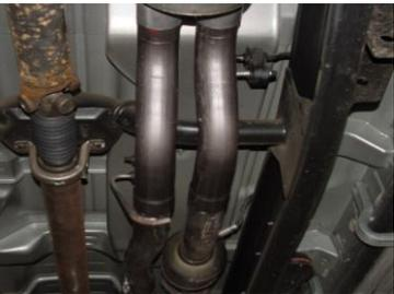
SLIDE PASSENGER SIDE HEADPIPE #A ONTO STOCK HEADPIPE. INSERT WELDED HANGER INTO RUBBER GROMMET. NEXT INSTALL DRIVERS SIDE HEADPIPE #B ONTO STOCK HEADPIPE, USE CLAMP #G TO SECURE BOTH HEADPIPES, DO NOT TIGHTEN.
