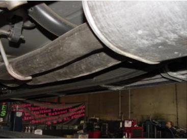
TO REMOVE STOCK EXHAUST, CUT 13" FROM THE FRONT OF THE MUFFLER, MEASURE TOWARDS THE FRONT OF THE VEHICLE. LEAVE ALL RUBBER GROMMETS ON THE HANGER. USE WD-40 TO AID IN THE REMOVAL OF EXHAUST AND HANGERS. SUPPORT THE CATALYTIC CONVERTER BEFORE CUTTING.
