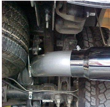
SLIDE EXIT PIPE # E ONTO OVERAXLE TAILPIPE INSERT WELDED HANGER INTO RUBBER GROMMET. USE CLAMP # I TO SECURE PIPES TOGETHER. DO NOT TIGHTEN. ROTATE PIPE UNTIL LEVEL.
