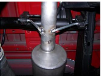
4. Slide the muffler #B into the headpipe at least 1.5"-2". Use a jack stand to support the muffler. Use clamp #E to secure muffler assembly to the headpipe. The outlet of the muffler will be at approximately 11 o'clock. The muffler inlet is looking into the louvers. Do not tighten.
