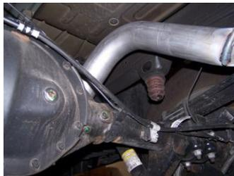
5. Slide tailpipe #C into muffler 1½"-2" and secure with clamp #F. Do not tighten. Insert welded hangers into rubber grommets.
