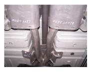
3. Install X pipe assembly #A assembly on to your front factory pipes and secure with factory clamps. Re-install factory cross member. Use a jack stand to support mufflers. Do not tighten.
