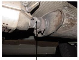
CUT 1" OFF BEHIND THE CONVERTER SO THE NOTCH IN THE MUFFLER WILL SLIP ON COMPLETELY.
