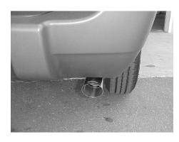
**INSTALL YOUR** STAINLESS TIP TO YOUR DESIRED LOOK. TO CLEAN TIP USE ANY ALUMINUM OR STAINI FSS CLEANER AND A SCOTCH BRITE PAD. NOW TIGHTEN ALL CLAMPS STARTING FROM THE FRONT AND WORKING BACK.
