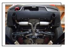
5. Install the supplied Tips (Item F) and leave them slightly loose for adjustment. Adjust the rest of the system for optimal fitment and clearance and tighten all clamps and bolts moving from front to back of the exhaust system.
