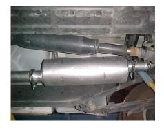
THEN INSTALL THE MUFFLER ON HEADPIPE #A NO LESS THAN 1-1/2" TO 2" USING CLAMP #E. THE MUFFLER OUTLET WILL BE CLOCKED AT 12 O'CLOCK POSITION. INLET OF MUFFLER HAS LOUVERS FACING THE MOTOR. DO NOT TIGHTEN.
