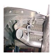
INSTALL WELDED HANGER INTO GROMMET.
