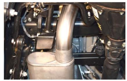
2. Install Item# A onto the factory Y-pipe re using the OEM Gaskets. Use the provide bolt kit Item G to secure the flanges to the factory pipes. Do not tighten.
