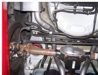
6. Now do the same procedure for the driver side tailpipe #B. Use clamp #E to secure the tailpipe to the muffler assembly and the stock clamp to secure it to the stock h-pipe.
