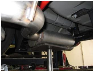
3. Now install the passenger side muffler assembly #B by sliding the metal hangers into the rubber grommets. Then do the same for the driver side muffler assembly #A. Use clamp #D to secure together.
