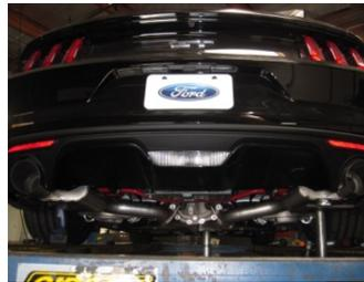
5. When you have everything in Place, firmly tighten all bolts And clamps down securely Use stainless steel cleaner and weekly to prevent tip from discoloration. Inspect all fasteners after 25-50 miles of operation and re-Tighten as necessary
