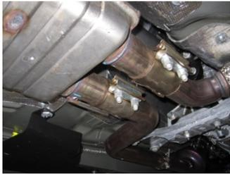
1. To remove your stock exhaust, unbolt it from the clamps located just after the manifolds then remove the whole exhaust system
