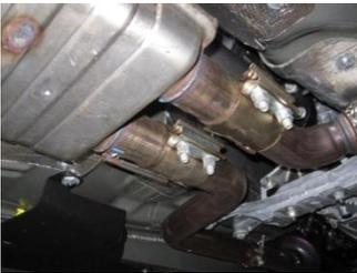
2. To remove your stock exhaust, unbolt it from the clamps located just after the manifolds then remove the whole exhaust system
