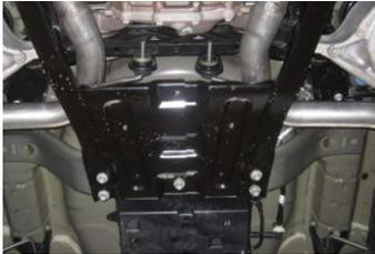
1. Prior to removing your factory exhaust you will need to remove the factory exhaust directly behind the rear diff and runs outward towards each vehicle door. There is a combined 8 bolts that need to be removed.
