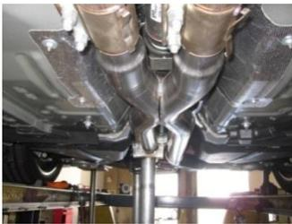
2. Install your Gibson x-pipe using the stock clamps. Be sure to keep loose until the entire system is in place.
