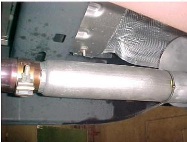
INSTALL HEADPIPE # A INTO STOCK PIPE. THE END OF THE PIPE SHOULD BE AT THE 9 O'CLOCK POSITION, ATTACH TO FACTORY CLAMP. DO NOT TIGHTEN.
