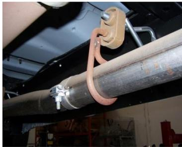
1. LAY OUT THE EXHAUST SYSTEM SO IT MATCHES THE DRAWING. MAKE SURE ALL PART NUMBERS ARE CORRECT. UNBOLT THE WELDED MUFLER ASSEMBLY IN FRONT OF THE MUFLER. DO NOT REMOVE THE EXTENSION PIPE BEHIND THE CONVERTER. FOR AN EASIER REMOVAL OF THE FACTORY EXHAUST. CUT THE TAILPIPE JUST BEHIND THE FACTORY MUFLER. LEAVE ALL RUBBER GROMMETS IN PLACE. USE WD-40 FOR EASIER REMOVAL OF FACTORY HANGER.
