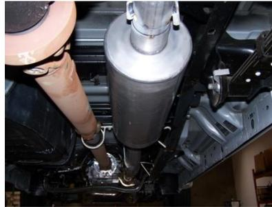
3. INSTALL MUFLER # B. THROUGH BAND CLAMP THEN SLIDE ONTO HEADPIPE 1 1/2" TO 2". USE CLAMP #E TO SECURE MUFLER TO HEADPIPE.
