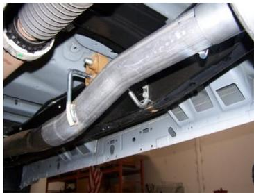
2. INSTALL HEADPIPE #A ONTO THE FACTORY EXTENSION PIPE. INSERT WELDED HANGER INTO RUBBER GROMMET. USE CLAMP #E TO ATTACH IT TO THE FACTORY EXTENSION PIPE. DO NOT TIGHTEN
