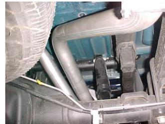
Install passenger side overaxle tailpipe #D into muffler 1 1/2" to 2". Secure with clamp #I. Do not tighten.
