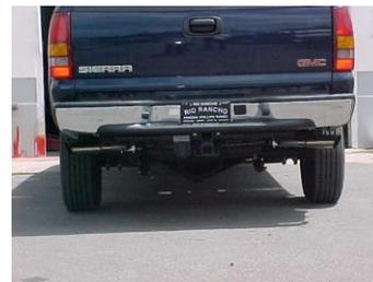
Install exit pipes #F. Use clamps #I to secure exit pipes to tailpipes. These clamps also attach to the metal hangers. Rotate to adjust for clamping. Now go back and tighten up all clamps, nuts, and bolts.
