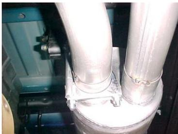
Next, install rear muffler hanger #H onto driverside muffler outlet and insert hanger into rubber grommet. Do not tighten.
