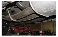
TO REMOVE STOCK EXHAUST, CUT 13" FROM THE FRONT OF THE MUFFLER, MEASURE TOWARDS THE FRONT OF THE VEHICLE. LEAVE ALL RUBBER GROMMETS ON THE HANGERS. USE WD-40 TO AID IN THE REMOVAL OF EXHAUST AND HANGERS. SUPPORT THE CATALITIC CONVERTER BEFORE CUTTING.
