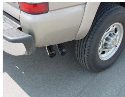
INSTALL YOUR BLACK CERAMIC COATED TIPS. PROCEED TO THE NEXT SHEET ON HOW TO INSTALL YOUR DEEGAN 38 BADGES. AFTER YOU HAVE CHECKED FOR CLEARANCES GO BACK AND TIGHTEN ALL NUTS, BOLTS AND CLAMPS.
