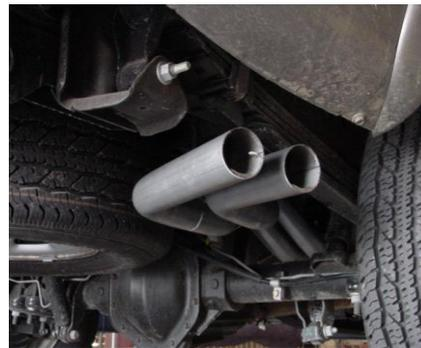
USE BOLT KIT #J TO SECURE TAILPIPES TOGETHER. THE PASSENGER SIDE TAILPIPE WILL BE ON THE BOTTOM.
