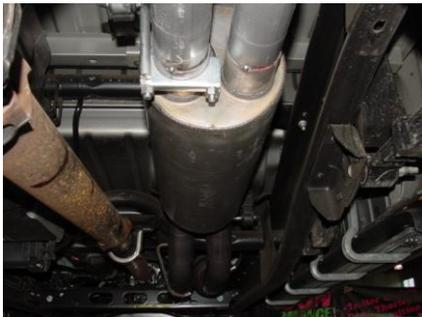
SLIDE MUFFLER #C ONTO HEADPIPES 1-1/2" TO 2". OUTLETS SHOULD BE AT THE BOTTOM. USE A JACK STAND TO SUPPORT MUFFLER AND ATTACH TO HEADPIPES WITH CLAMP #G.
