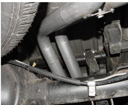
SLIDE PASSENGER SIDE TAILPIPE #E INTO MUFFLER 1-1/2" TO 2". USE CLAMP #I TO SECURE TAILPIPE TO MUFFLER. DO NOT TIGHTEN.
