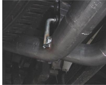
SLIDE DRIVERS SIDE TAILPIPE #D INTO MUFFLER 1-1/2" TO 2". INSERT WELDED HANGER INTO RUBBER GROMMET.
