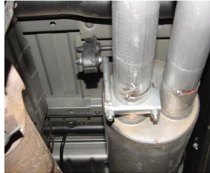
INSTALL HANGER #H INTO RUBBER GROMMET JUST ABOVE DRIVERS SIDE OF MUFFLER OUTLET. YOU WILL USE THIS CLAMP TO SECURE TAILPIPE TO MUFFLER, DO NOT TIGHTEN.
