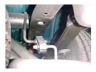
Install drivers side over axle tailpipe #C into muffler and secure pipe to muffler using clamp #G. Insert welded hanger into rubber grommet.
