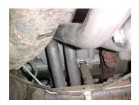
Install passenger side over axle tailpipe # C into muffler and attach using clamp # H. Use bolt kit # I to attach the tailpipes together. Insert hanger into rubber grommet. Do not tighten. YOU MAY NEED TO LOOSEN YOUR SPARE TIRE & PUSH TOWARDS DRIVER SIDE & RE-TIGHTEN.
