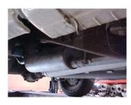
Install muffler #B onto head pipe # A 1-1/2" to 2" with the louvers facing towards the converter. Use a jack stand to support the muffler. Use clamp # G to secure the muffler to the head pipe. Do not tighten.
