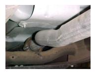
Lay out the exhaust on the floor so it looks like the drawing and compare parts with manual. To remove the stock exhaust un-bolt it from the flange located in front of the muffler. You will re-use your stock hardware. Leave all rubber grommets in place. Use WD-40 to aid in removal of the hangers. Cut your stock tailpipe off just behind the muffler for easier removal.
