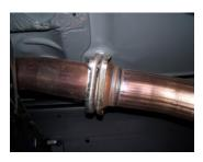
**2.** To remove the stock exhaust, unbolt the head pipe at the 2 bolt flange. Disengage the welded hangers using WD-40 from the OEM rubber grommets. Do not damage or remove the rubber grommets as you will reuse them to mount your new system.
