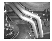
NOW INSTALL DRIVERSIDE TAILPIPE #D. THE SPARE TIRE MAY NEED TO BE LOOSENED AND PUSHED TO THE DRIVER SIDE TO ALLOW FOR CLEARANCE. USE BOLT KIT # I TO ATTACH BOTH TAILPIPES TOGETHER. DRIVERSIDE TAILPIPE BRACKET WILL BE POSITIONED ON TOP OF PASSENGER TAILPIPE BRACKET.
