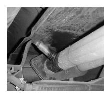
Remove O2 sensor from stock head pipe and remove stock flange gasket. You will reuse the stock bolts.
