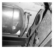
Unbolt stock flange behind the rear of the converter. You will reuse the stock bolts. Remove stock hangers leaving rubber grommets in place. Use WD-40 on hangers for easier removal. Cut & remove the stock tailpipe.
