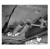
Bolt head pipe #A to the stock head pipe flange behind the converter reusing stock bolts and supplied gasket. Use a Hi-Temperature 02 sensor safe silicone on the gasket for a good seal. Insert welded hanger into rubber grommet. Re-install 02 sensor into head pipe. Apply a small amount of anti-seize on the threads. Do not tighten.
