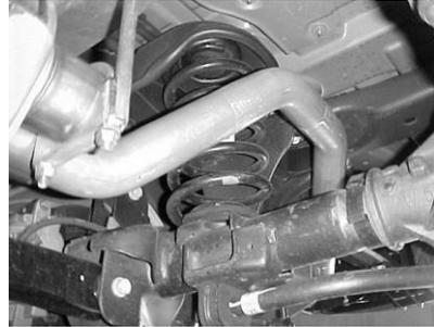
INSTALL PASSENGER TAILPIPE #D INTO MUFFLER OUTLET NO MORE THAN 1-1/2" TO 2". INSERT THE WELDED HANGER INTO THE RUBBER GROMMET. USE CLAMP # G TO ATTACH TO MUFFLER OUTLET. DO NOT TIGHTEN
