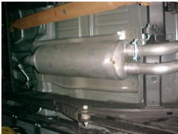
INSTALL MUFFLER # B ONTO HEAD PIPE 1-1/2"-2" WITH THE LOUVERS FACING TOWARDS THE CONVERTER. USE A JACK STAND TO SUPPORT THE MUFFLER. USE CLAMP # F TO SECURE THE MUFFLER TO THE HEADPIPE. DO NOT TIGHTEN.
