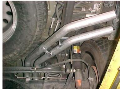
ATTACH BOTH TAILPIES USING BOLT KIT # I. THE PASSENGER SIDE MOUNTING BRACKET WILL BE POSITIONED UNDERNEATH THE DRIVERSIDE. NOW GO BACK AND TIGHTEN ALL CLAMPS, HANGERS AND BOLTS.
